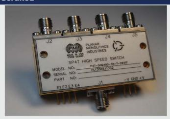
PMI Model No. P4T-50M40G-55-T-292FF is a 50MHz to 40.0GHz, Single Pole, Four Throw, Absorptive Switch. This switch offers 55dB of port to port isolation and a maximum insertion loss of 8db. It has a switching speed of 100ns and is independently TTL controlled. The operating power is +20dBm CW and it has a VSWR of 2.5:1 max.
